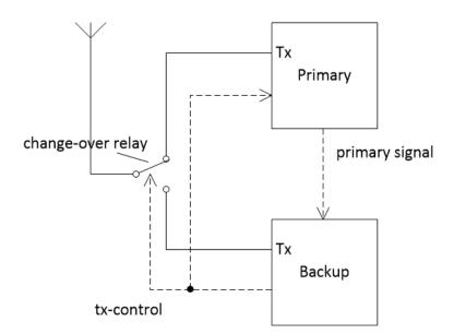
The backup supervises the primary by means of a digital signal from the primary, which indicates whether the primary is up (nominal) or down (failed).
