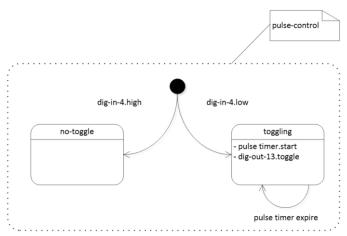
The program logic has two states. When digital input 4 is high, the no-toggle state does nothing interesting. When digital input 4 is low, a toggling state uses a timer to toggle digital output thirteen.
